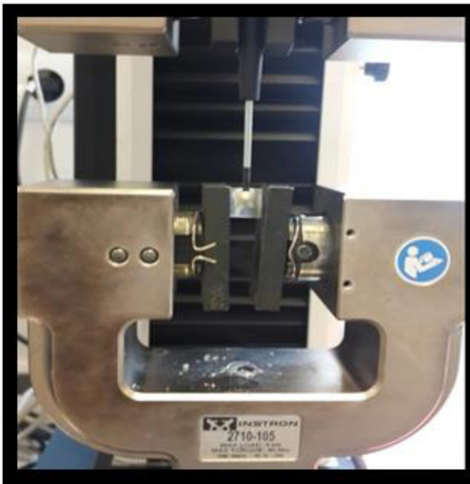
Figure 3. Instron universal test device and a sample put into the device
