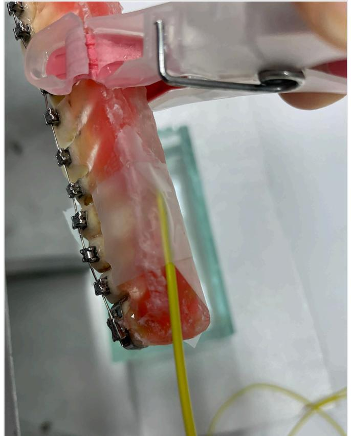
Figure 4. Thermometer tip placement within the root
