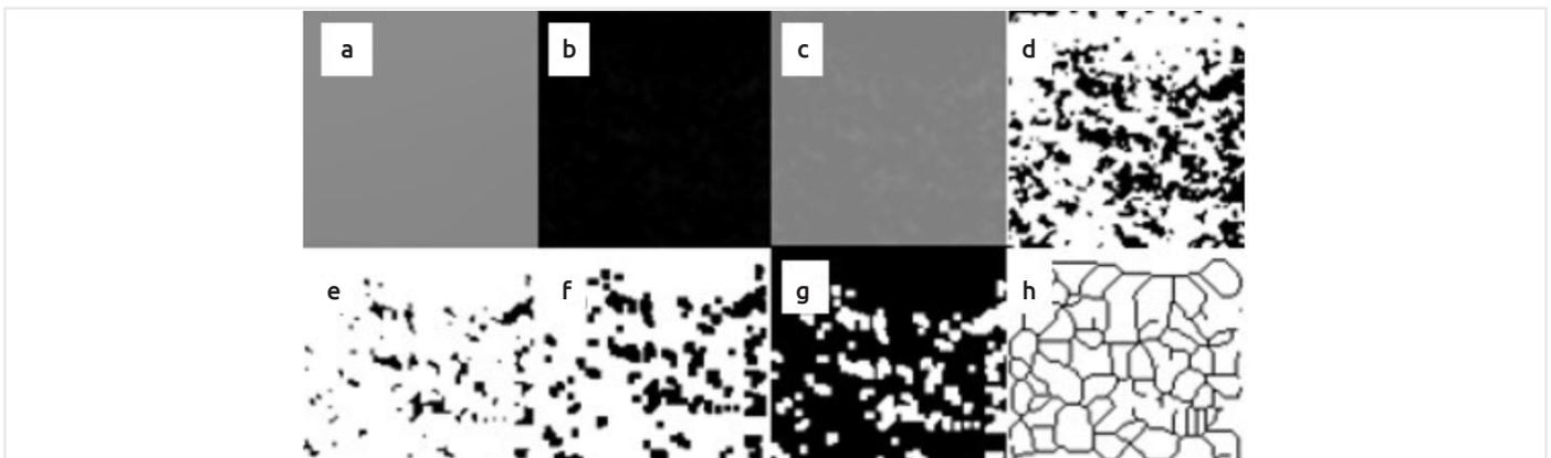
**Figure 2.** a) Blurring; b) Removing the blurred image from the original image; c) Adding 128 shades of gray; d) Black-and-white image conversion; e) Noise reduction with Erode; f) Expansion with Dilate; g) Color inversion; h) Convert to skeletal format
